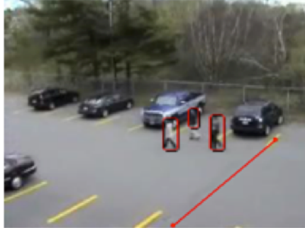
Trip wire will alert operators when people or objects enter into a specific field of view.
