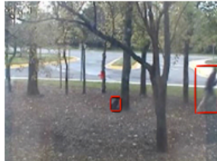
Video analytics will send an alert when suspicious objects are left behind in a field of view.
